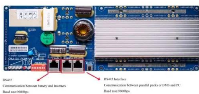
RS485 Communication between battery and inverter Baud rate: 9600bps RS485 Interface Communication between parallel packs or EMS and PC Baud rate: 9600bps
